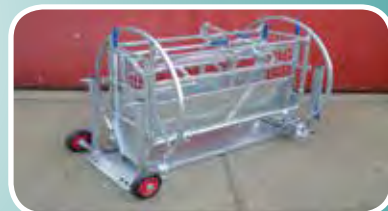
Turning crate sideways for hoof trimming
