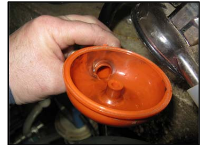
Fig. 38. Inking from rubber breakdown
