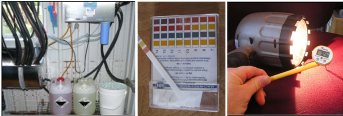
Fig. 24. Left - verify cleaners used correctly; Middle - pH paper to check acidity / alkalinity; Right - thermometer and strong flashlight
