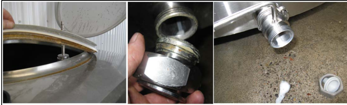
Fig. 41. Milk tank equipment needs to be inspected and cleaned after every pick-up
