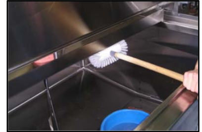
Fig. 19. Manually clean bulk tank
