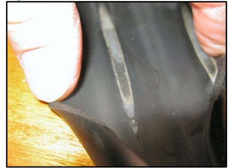
Fig. 20. Liner cracks with bacteria
